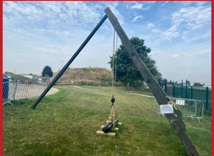
A replica Gyn lift is constructed complete with tackle
